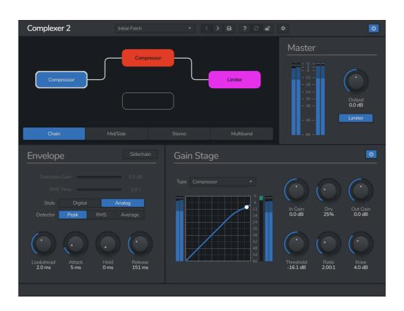
Complexer 2 is a multi-stage dynamics processor, featuring three independently controlled dynamics processors, each with a choice of six different modes.
